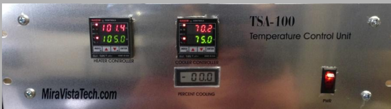
Remote temperature control unit
