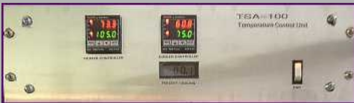
Remote temperature control unit
